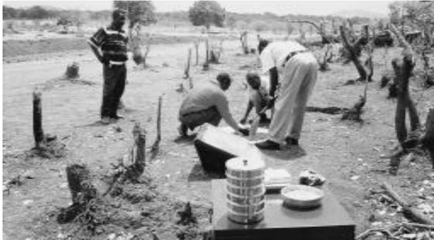
Soils testing kit used for in-situ materials testing on site
